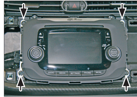
6. Remove 4 screws of head unit (see arrows)
