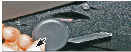
2. Open glove box. Unclip and remove cover under dash board (see arrow)
