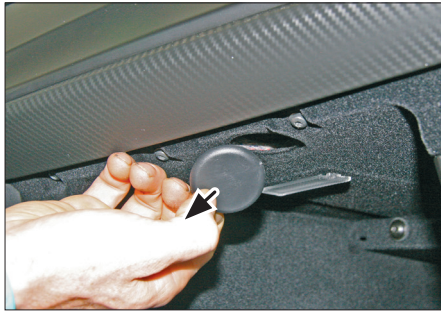
2. Open glove box. Unclip and remove cover under dash board (see arrow)
