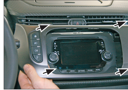
5. Unclip and remove center panel (remove plugs carefully!)
