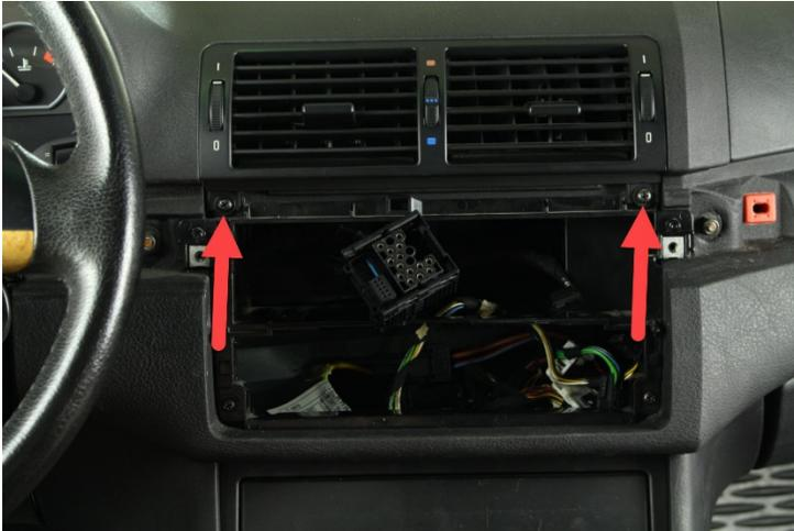
7. Use a Phillips screwdriver to remove the screws securing the ventilation slots.
