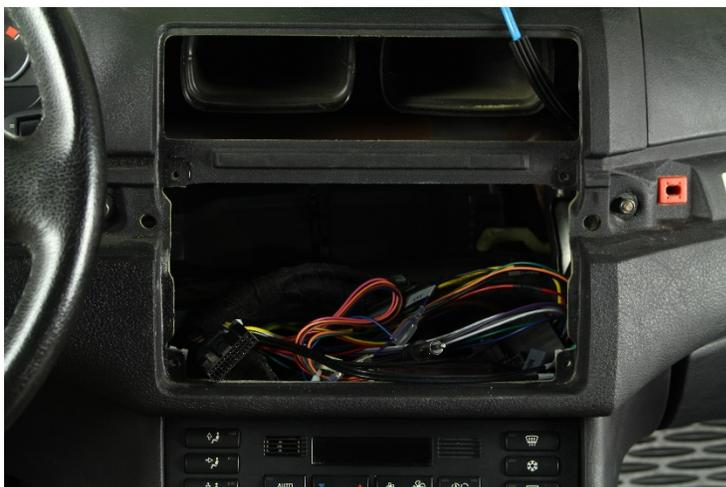
13. Connect the main harness (# 11/12) of the Radical device (# 1) to the plug of the vehicle and close the locking mechanism of the connector. Then connect the CAN bus interface (No. 13) to the main harness. Connect all cables previously routed in the radio slot and the original antenna cables to the Radical unit (# 1)
