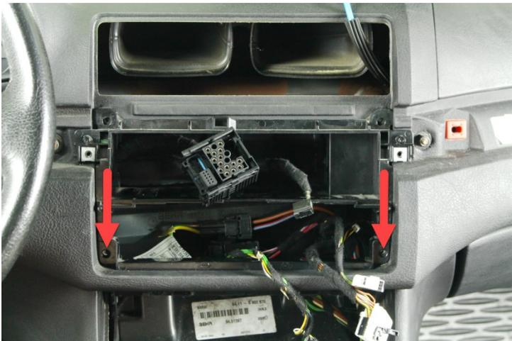
9. Loosen the last two screws securing the plastic frame and carefully remove it from the radio bay.
