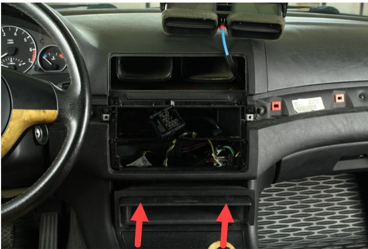
8. Open the storage compartment underneath the radio bay and use a screwdriver to loosen the screws of the storage compartment.
