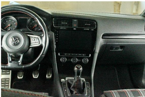
11. Neatly arrange the wires to the side, making room for the Radical device. Carefully slide it into the radio slot. Push back the R-C10VW2 until you hear the clicking sound of the latching mechanism.
