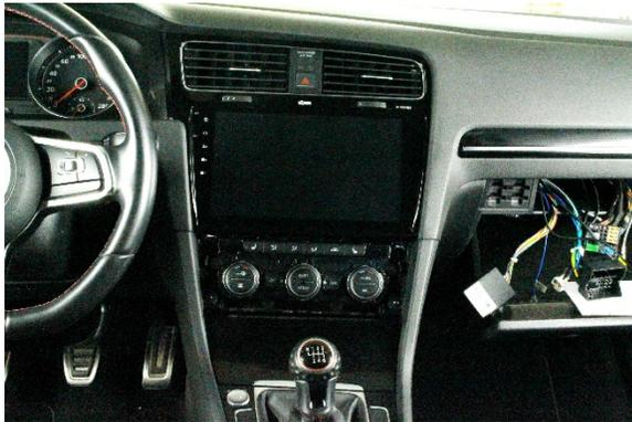
10. Connect one of the main connection cables (No. 11) of the Radical device (No. 1) to the Plug connector of the car and close its locking mechanism. Following this, connect the CAN bus interface (No. 12) to the main connection cable. Connect all the cables inside the radio bay and the original antenna cables.
