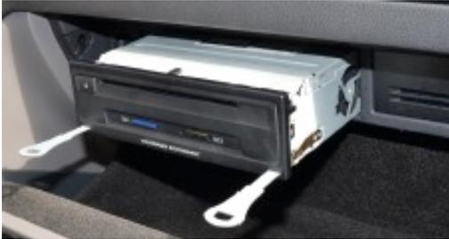
7. If your vehicle is equipped with an external control module for the infotainment system, you have to remove it first. Use the removal tools to pull out the module, unlock all connectors on the backside and remove it completely.
