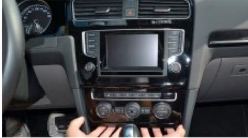
1. Open the lid of the ashtray approx. half to access and manually remove the bezel of the air-conditioning panel.
