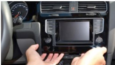
2. Pull the radio frame panel on the lower part forward to unlock it from the multimedia operating panel.
