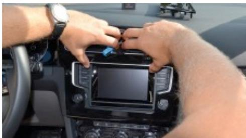
5. Reach into the opening of the removed head unit to jerk the radio front panel forward. During removing the radio front panel, please pay attention to release the connection assemblies of the radio front panel at the transition to the instrument cluster carefully.
