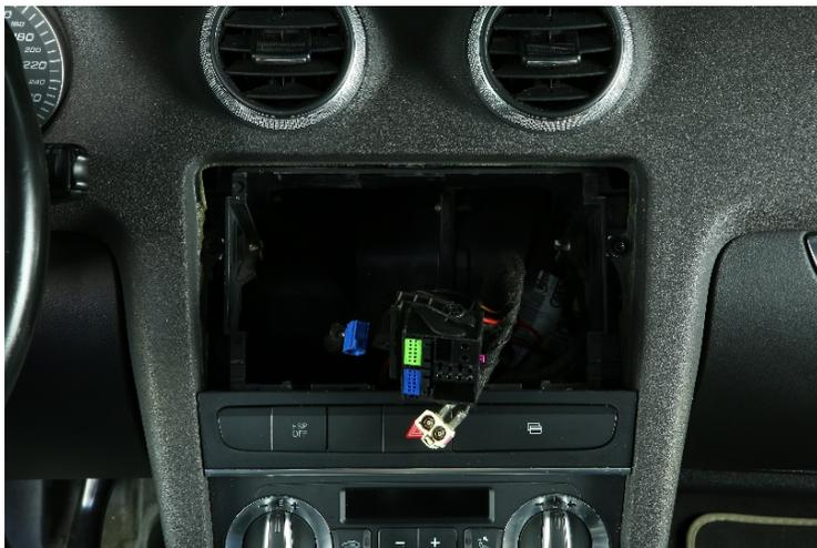
3. To completely remove the OE radio, all the cables (i.e. main harness, antenna cable etc.) must be unplugged on the backside of the device. Put the radio aside in a safe place, to protect it from damage.
