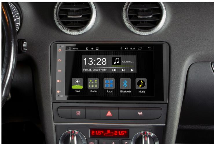
7. Neatly arrange the wires to the side, making room for the Radical device. Carefully slide it into the radio slot. Push back the R-C11AD1 until you hear the clicking sound of the latching mechanism. The installation of your R-C11AD1 is now complete.
