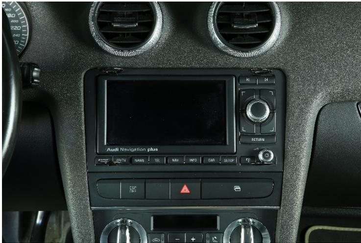
1. Unlock the OE factory radio with the unlock tool (No. 17) contained in the set. You need to insert all four keys.
