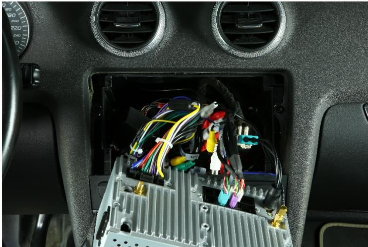
6. Connect one of the main connection cables (No. 11/12) of the Radical device (No. 1) to the Quadlock/ISO connector of the car and close its locking mechanism. Following this, connect the CAN bus interface (No. 14) to the main connection cable. Connect all the cables to the Radical device (No. 1) those previously run in the radio slot, and the original antenna cables.
